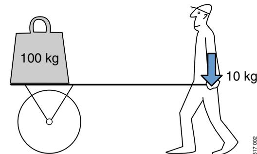
The load for the person varies in relation to the position of the load on the trolley.
